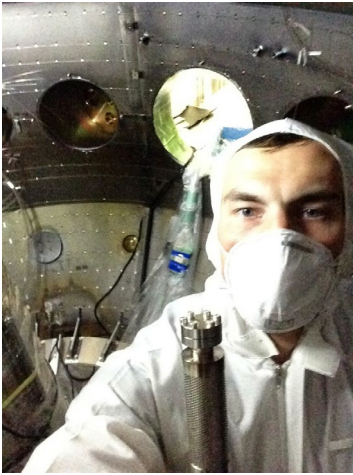
Fig. 5. During Permeation Probe installation, inside QUEST tokamak.
